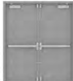
Both Doors Active w/ Surface Vertical Rod Exit Devices
